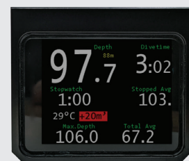
Digital bottom timer with 63mm (diagonal) display
